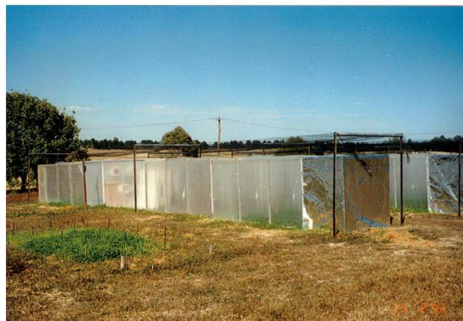
Figure A9.1. Temperature gradient tunnel imposing CO<sub>2</sub> and temperature treatments as described by Lilley *et al.* (2001). Photograph J. Lilley.
